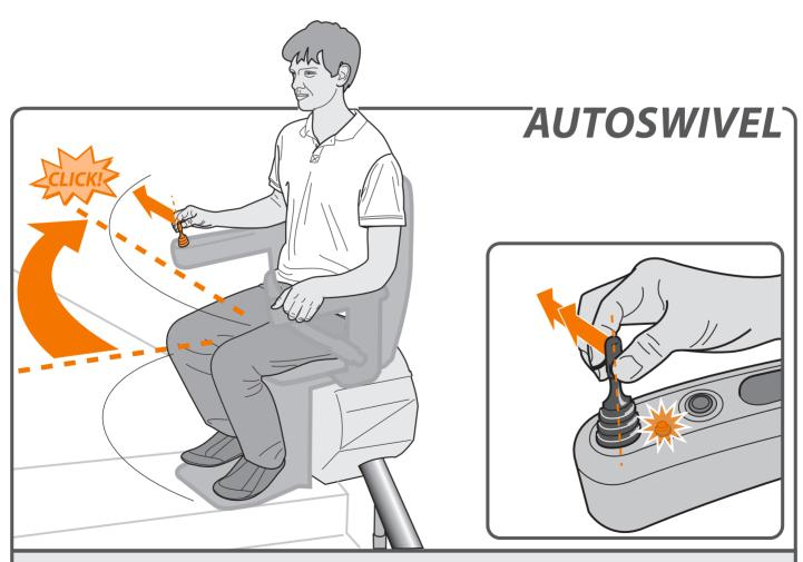
The AUTOMATIC SWIVEL SEAT option let you swivel the seat automatically to face the direction you are going to walk in. To do this, push and hold the joystick in the upwards direction.
