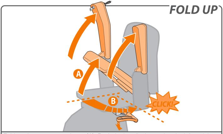
Fold up the armrests and seat {A}. Push the handle, located to the left or right under the seat, downwards. Swivel the seat until you hear a 'click'. The seat is now in the locked position {B}.
