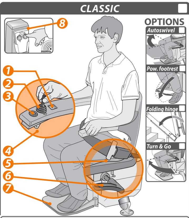
The illustration opposite shows the features used to operate the Classic seat. The Classic can be upgraded with the automatic swivel seat, powered footrest, hinged rail and Turn & Go options to create even more seat comfort and user-friendliness.
