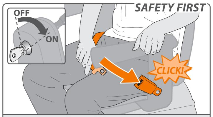
Fasten the seat belt securely, ensuring that it clicks into the holder. Put the key in the switch and turn it ninety degrees clockwise. The LED on the armrest lights up faintly.
