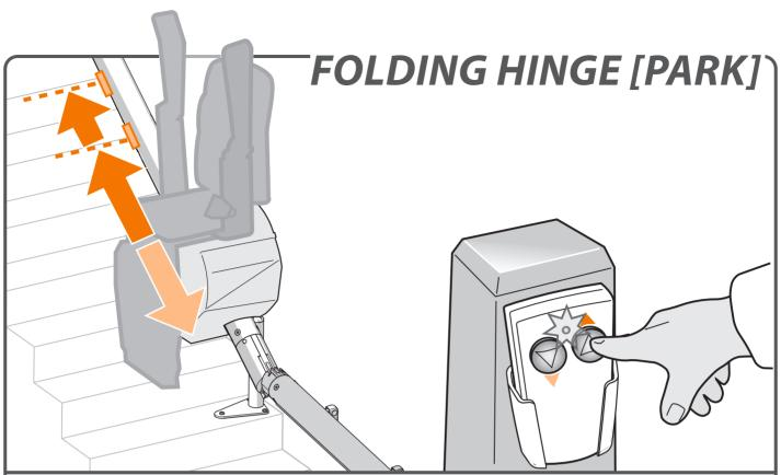
Do not leave the lift on the hinged rail after use. Use the remote control to move the lift to a charge point and recharge the batteries. The first stopping point is at the hinged rail. Keep moving the lift until it reaches a charge point further up.
