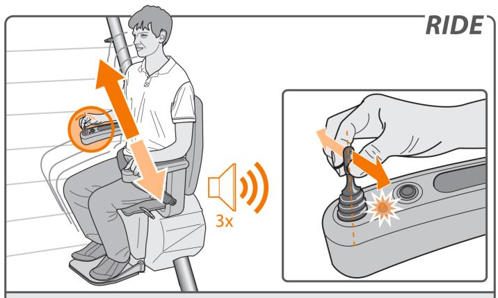
Move the joystick in the desired direction of travel. The LED lights up. The lift beeps three times, then gradually starts to move.
