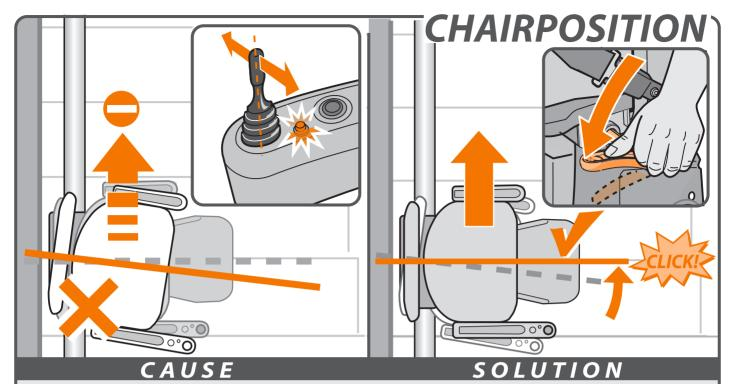
**Problem:** the lift does not travel in either direction and the LED flashes when the joystick is operated.
