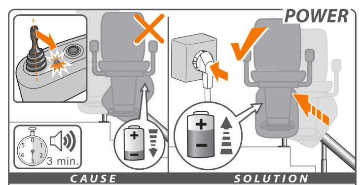
Problem: the lift batteries are not recharging, the LED is flashing and the lift beeps for three minutes.
