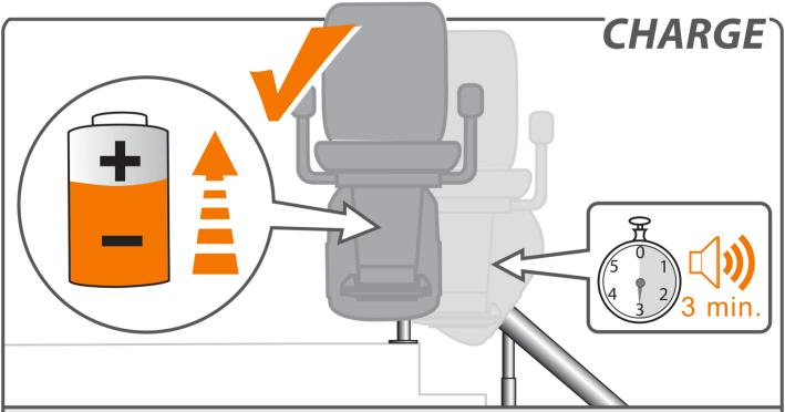
There are charge points for recharging the lift's batteries at the top and bottom of the rail (there may be additional charge points). If the lift is not in the correct position at the charge point, the lift beeps for three minutes and the LED in the armrest flashes. The lift does not work if the batteries are flat.
