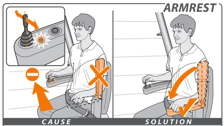
**Problem:** the lift does not travel in either direction and the LED on the armrest lights up when the joystick is operated. **Cause:** an armrest has not been folded down. **Solution:** fold down the armrest fully.
