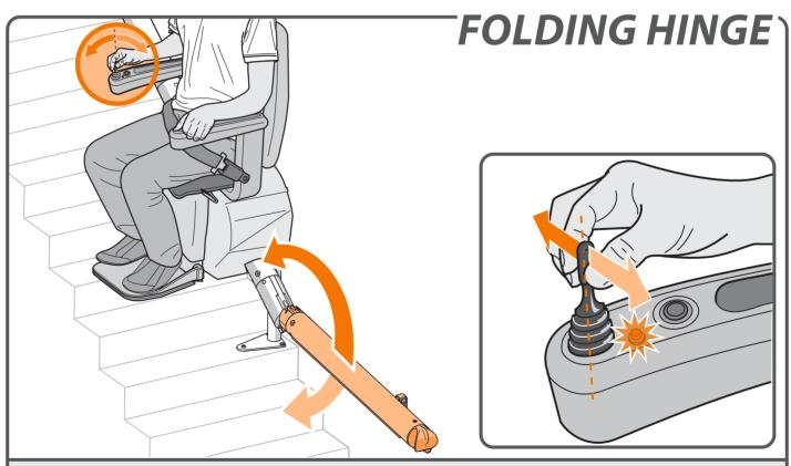
With the FOLDING HINGE option, the seat stops just above the hinged rail. Move the joystick up or down to fold or unfold the rail.
