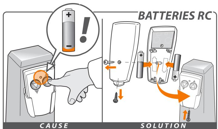
**Problem:** the lift does not travel in either direction and the LED on the remote control does not light up when the remote control is operated.
