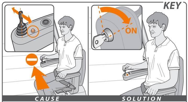
**Problem:** the lift does not travel in either direction and the LED on the armrest does not light up when the joystick is operated.
