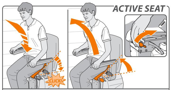
With the ACTIVE SEAT option, the seat assists you when sitting down and standing up. To stand up, pull the handle, located to the left or right under the seat, upwards. The seat pushes you up. When you sit back down, the seat slowly returns to its normal position and clicks into place.
