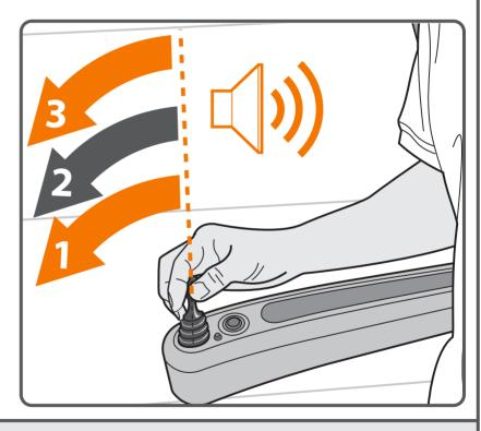
Stairlift with powered swivel can swivel automatic on a preferent intermediate landing after tapping. Before the start of the lift, the joystick (not the remote control) is operated in the direction of travel (Tap). The number of operations (taps) indicates the desired floor. Tapping must be done rather quickly. After each tap you hear a beeping sound. LAST press (when holding the joystick to start driving) is NOT counted as a tap !!
