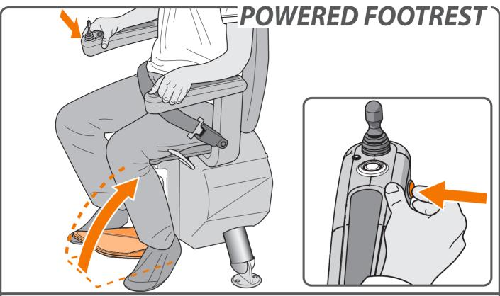
The POWERED FOOTPLATE option lets you fold the footplate up and down automatically using the switch on the side of the armrest. The footplate lights up when folded down.
