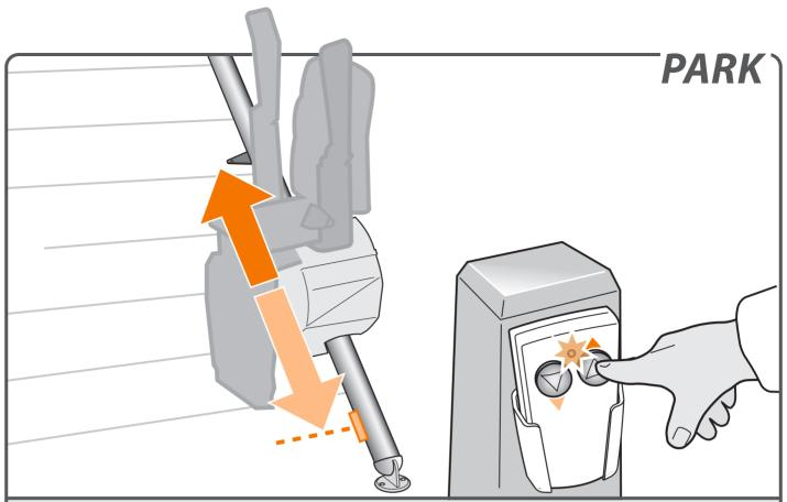
Press and hold the button on the remote control until the lift reaches a charge point. Upon arrival, the lift stops automatically and the LED on the remote control goes out.
