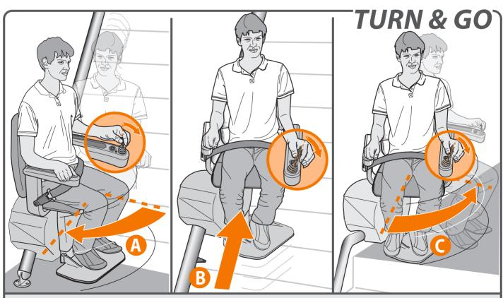
The TURN & GO option swivels the seat so that you travel up and down with your back to the stairs {B}. Hold the joy stick in the desired direction of travel, at the start and end of the rail {A and C}.
