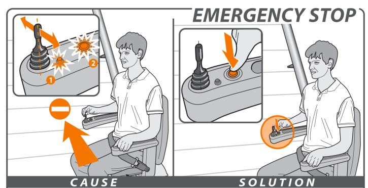
**Problem:** the lift does not travel in either direction, the LED[1] flashes when the joystick is operated and the emergency stop [2] is illuminated.
