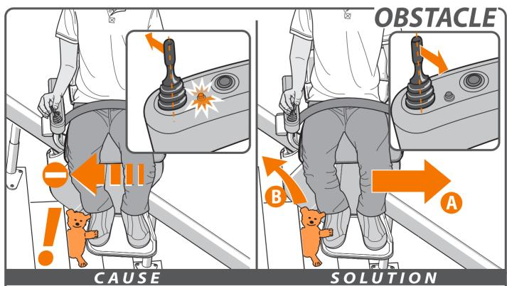
Problem: the lift travels in one direction only and the LED flashes when the joystick is operated.
