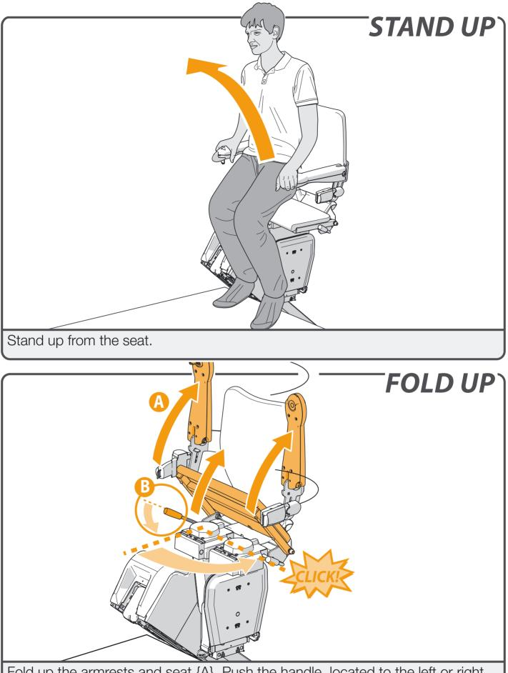
Fold up the armrests and seat {A}. Push the handle, located to the left or right under the seat, downwards {B}. Swivel the seat until you hear a 'click'. The seat is now in the locked position.
