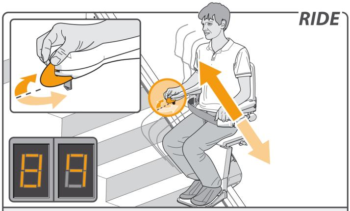
Move and hold the joystick in the desired direction of travel. The display shows a "**8/9**", the lift gradually starts to move.
