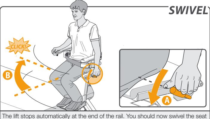
The lift stops automatically at the end of the rail. You should now swivel the seat manually, making it easier to get on and off. To do this, push down the lever{A}. Swivel the seat until you hear a 'click'. The seat is now in the correct position{B}.
