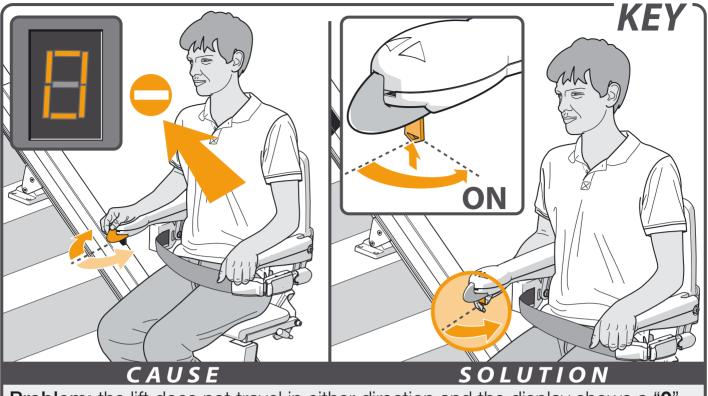
Problem: the lift does not travel in either direction and the display shows a "0".Cause: the key-operated switch is in the off position.Solution: turn the key-operated switch ninety degrees clockwise.
