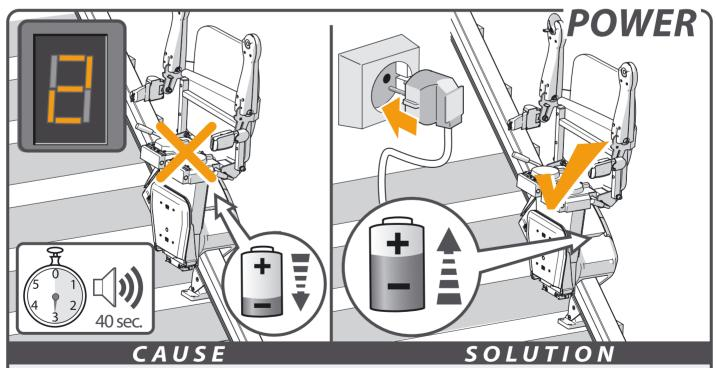
Problem: the lift beeps for 40 seconds and the display shows a "2".Cause: the lift batteries are not recharging, possibly the plug is not in the socket.Solution: put the plug in the socket.
