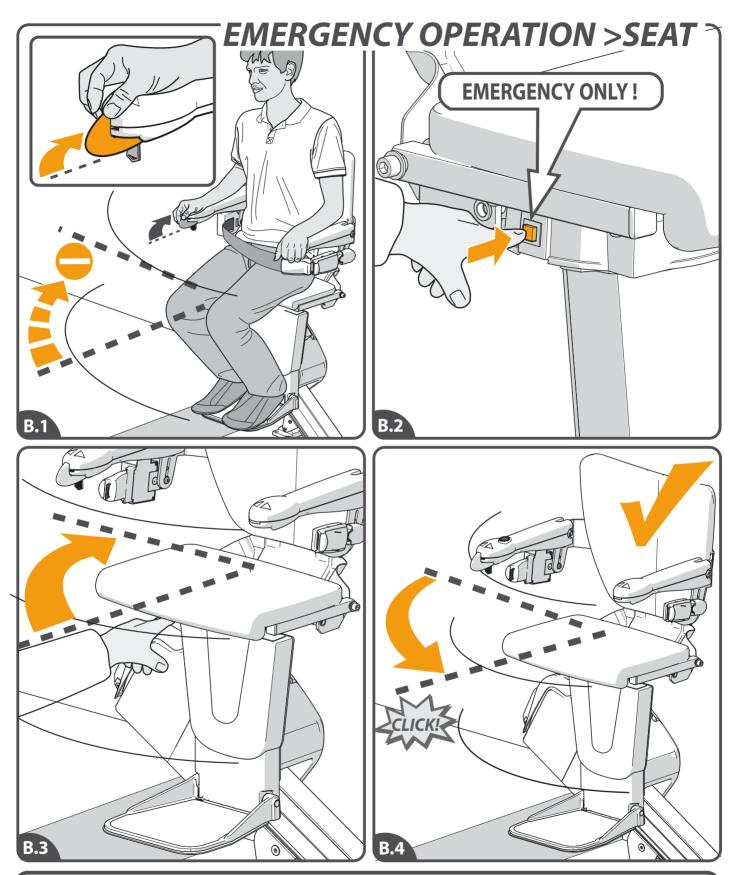
[B.1]If the powered swivel is not functioning it can be swivelled manually. Do this only in an emergency. [B.2]Press the release button. [B.3]Swivel the seat manually. [B.4]The seat must be returned to the start position.Do this before you use the lift again.
