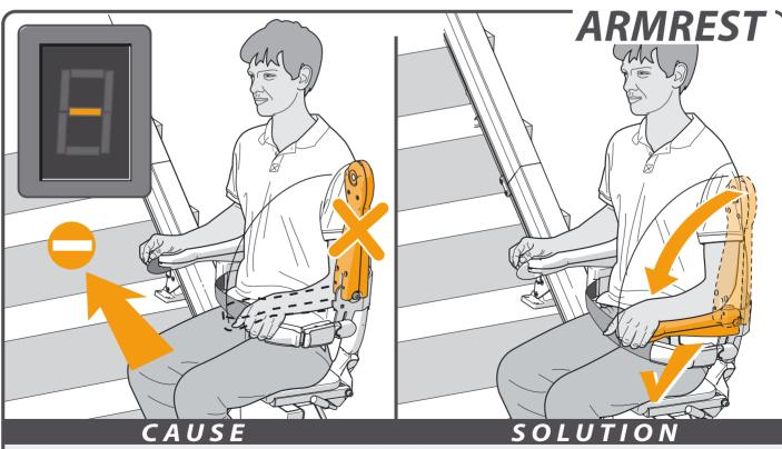
Problem: the lift does not travel in either direction and the display shows a "-".Cause: an armrest has not been folded down.Solution: fold down the armrest fully.
